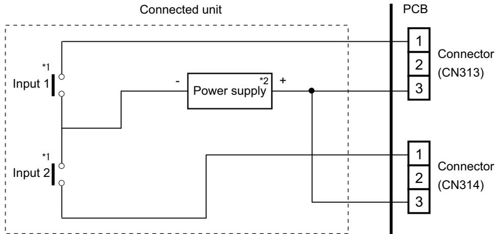
\*1: The switches can be used on the following condition: DC 12 V to 24 V, 1 mA to 15 mA.
