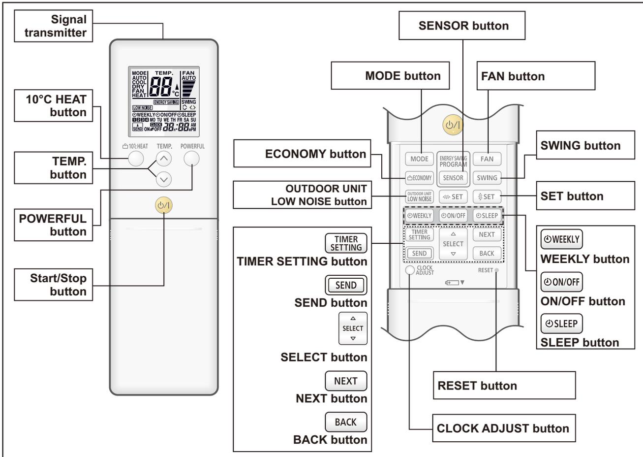
**NOTE:** Functions may differ by type of the indoor unit. For details, refer to the operation manual.
