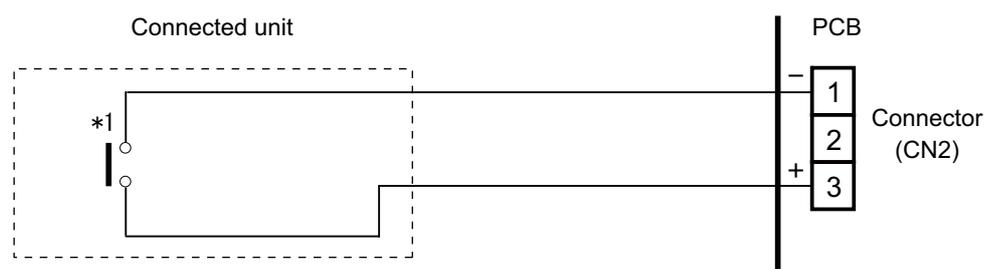
\*1: The switch can be used on the following condition: DC 12 V to 24 V, 1 mA to 15 mA.
