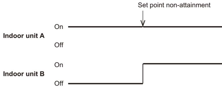
\*: Operation is started even when the unit is stopped by the weekly timer.
