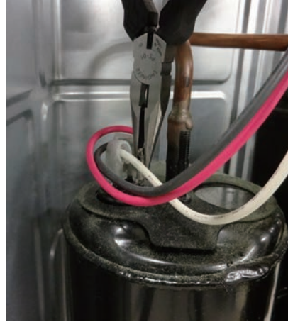
4. Remove the connectors. [ R : White, S : Red, C : Black ]
