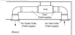
When connecting the duct, perform duct-insulation appropriate for the installing environment.
