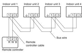
(2) Set the R.C. address (DIP switch setting)
