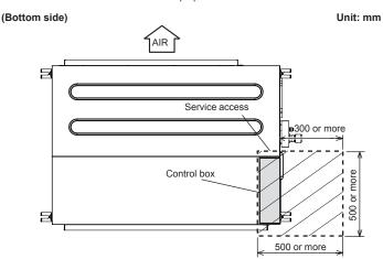
\* The service access necessary for fan units and filter maintenance
