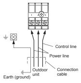
\*Ground the remote controller if it has a earth (ground) wire.
