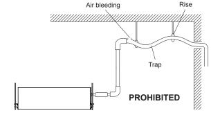
Observe the following procedures to construct centralized drain pipe fittings.
