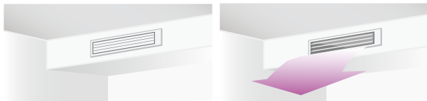
Closed louver [Operation is stopped.]
