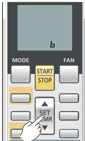
4. Press the MODE button again to return to the clock display. The custom code will be changed.
