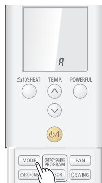
3. Press the TEMP. "↑" or the "↓" button to change the custom code between A → b → c → d.
