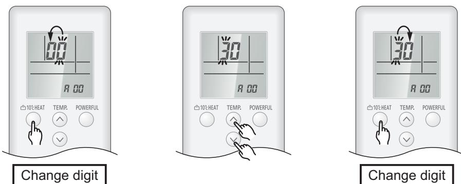
4. Proceed to the setting number by pressing the POWERFUL button. (To return to the function number selection, press the POWERFUL button again.)
