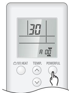
5. Select the function number by pressing the  $\wedge$  or the  $\vee$  button. Each time the  $10^\circ\text{C HEAT}$  button is pressed, it switches between the right digit and the left digit.
