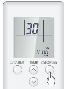
5. Select the function number by pressing the  $\wedge$  or the  $\vee$  button. Each time the  $10^{\circ}\text{C}$  HEAT button is pressed, it switches between the right digit and the left digit.
