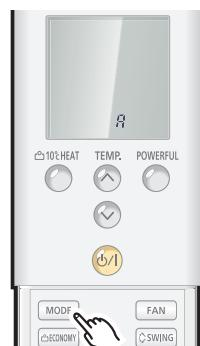
3. Press the SET TEMP. "▲" or the "▼" button to change the custom code between  $\text{A} \rightarrow \text{B} \rightarrow \text{C} \rightarrow \text{D}$ .
