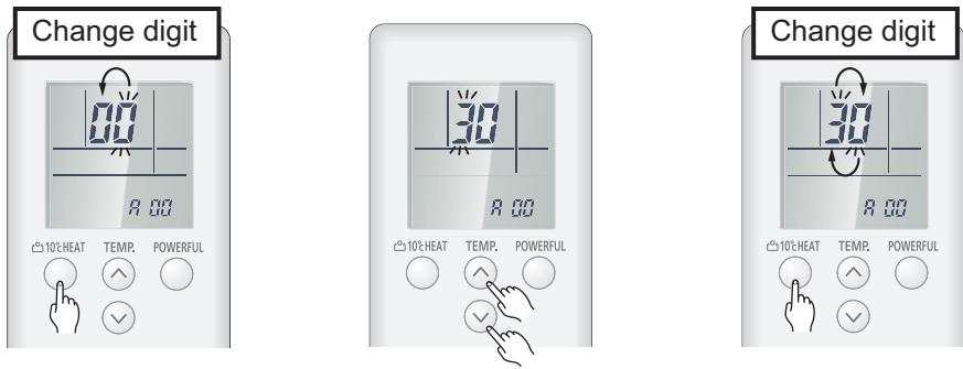
4. Proceed to the setting number by pressing the POWERFUL button. (To return to the function number selection, press the POWERFUL button again.)
